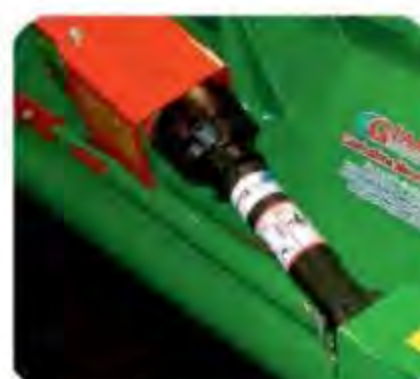
Mechanical transmission with oil-bath universal joint
