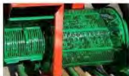
Rotary sieve for hazelnuts dia. Ø 26
