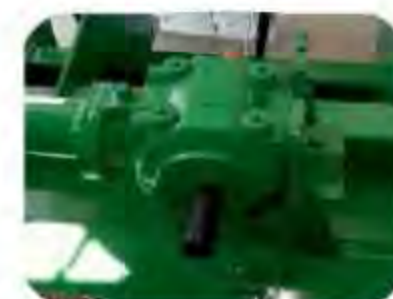
Rear PTO for reversible linkage or PTO connection of the inter-row disc.
